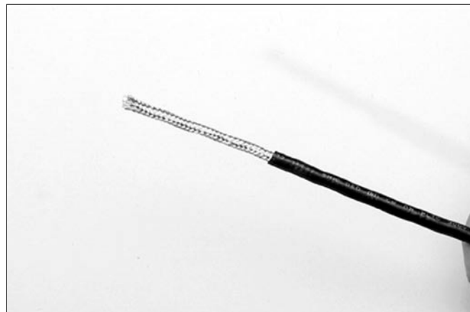
Figure 3.9 – Removing outer plastic jacket
