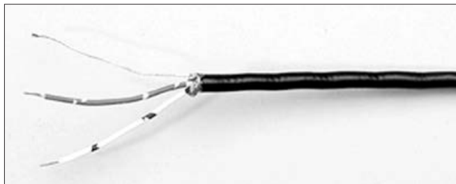
Figure 3.17 – Stripping conductors and applying heat shrink tubing
