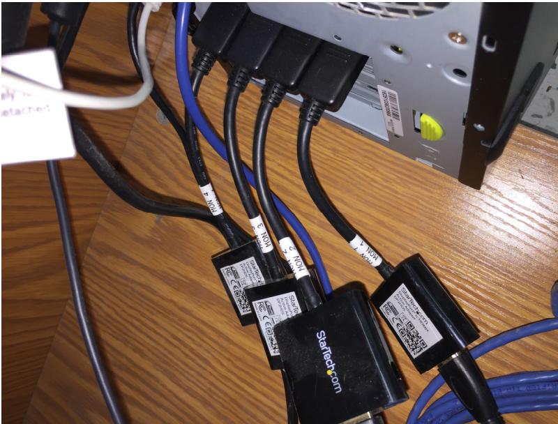
On Multi-Monitor Systems, Display Cables Should Be Marked For Easy Hookup
